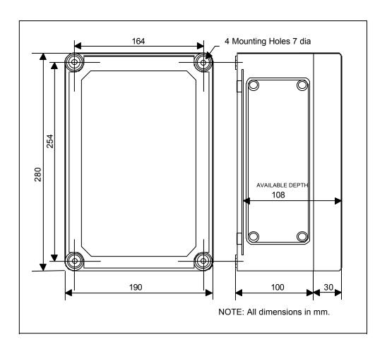
The Basic Enclosure is an impact resistant, polycarbonate enclosure which offers protection from dust and moisture in accordance with IP67 (IEC529/DIN 40050/BS5490). It is moulded from homogeneous thermoplastic polycarbonate, is resistant to normal atmosphere corrosion and is resistant to most mineral and organic acids. Contact should be avoided, however, with organic solvents and strong alkalis. The material is self-extinguishing and does not release any toxic combustion products.
